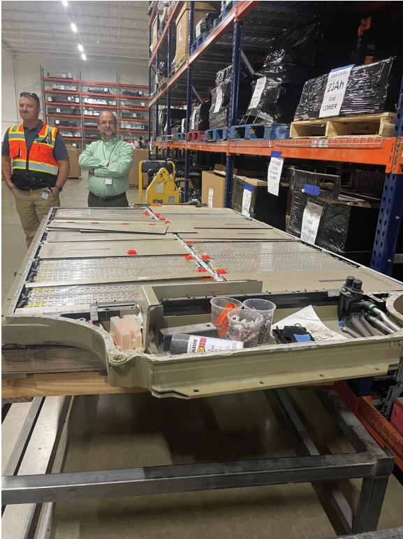
Figure 2. EV (Tesla) battery, not fully enclosed; individual cells secured to outer frame.
