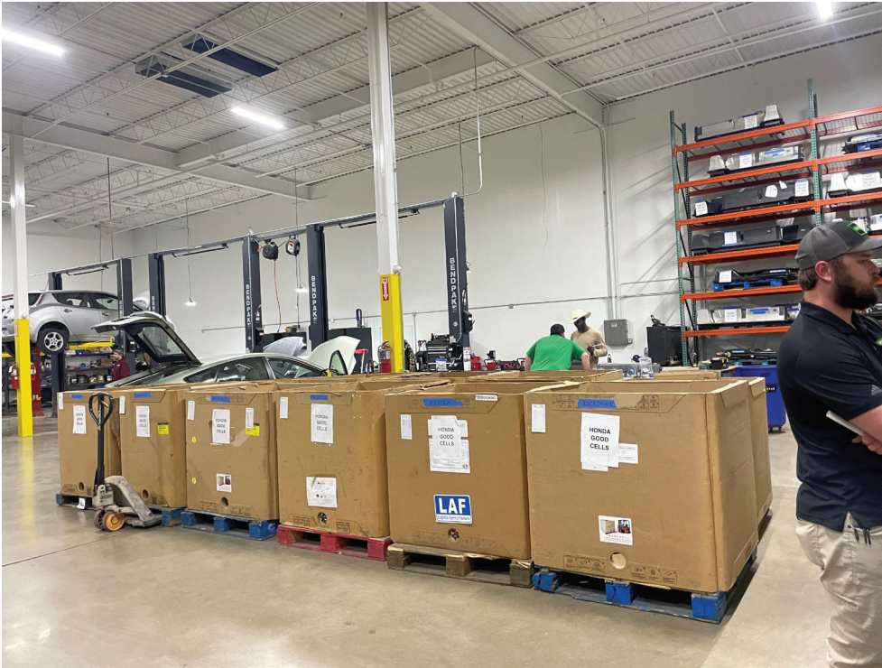
Figure 4. Sorting boxes with “good” cells that have been tested and separated from “bad” cells.
