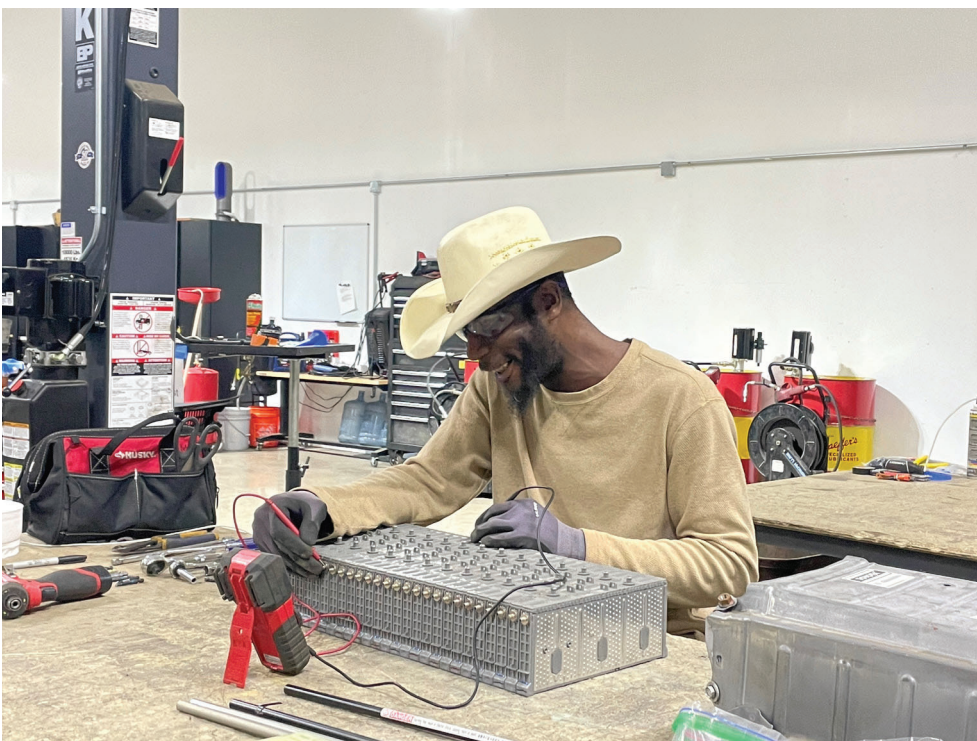
Figure 5. Greentec Auto technician testing individual cells for viability.
