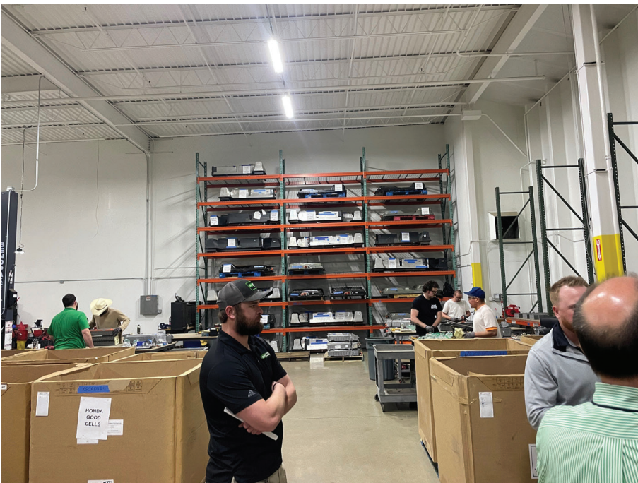
Figure 3. Disassembly, sorting, and testing room; boxes with “good” battery cells, shelving with reassembled batteries.
