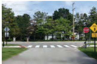
Shared Use Sidepath. Nall Avenue path accommodates travel in both directions. Warning signs for motorists and high visibility crosswalks at street crossings will add to the safety of these facilities
