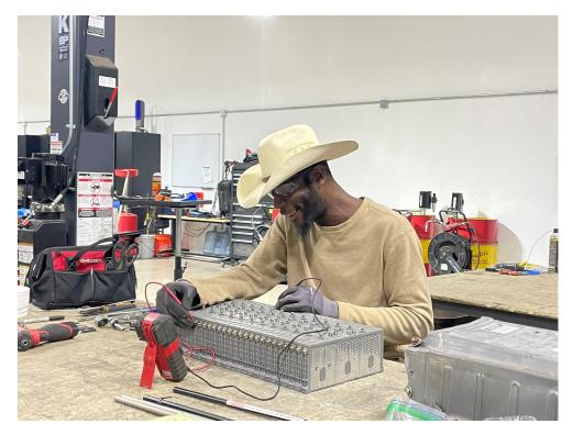
Figure 5. Greentec Auto technician testing individual cells for viability.
