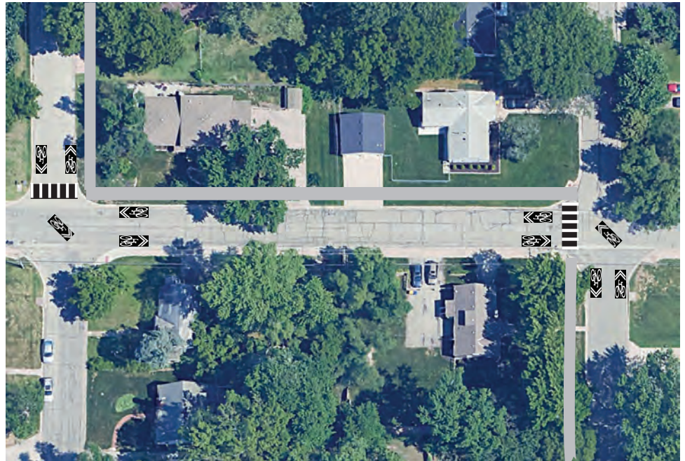
Negotiating jogs in the route. The Maple/Reed bicycle boulevard includes several jogs because of disconnected or offset streets. These can be addressed through short sidewalk or sidepath segments on the busier connecting street and crosswalks. Shared lane markings can be used here to guide on-street cyclists through the jog.
