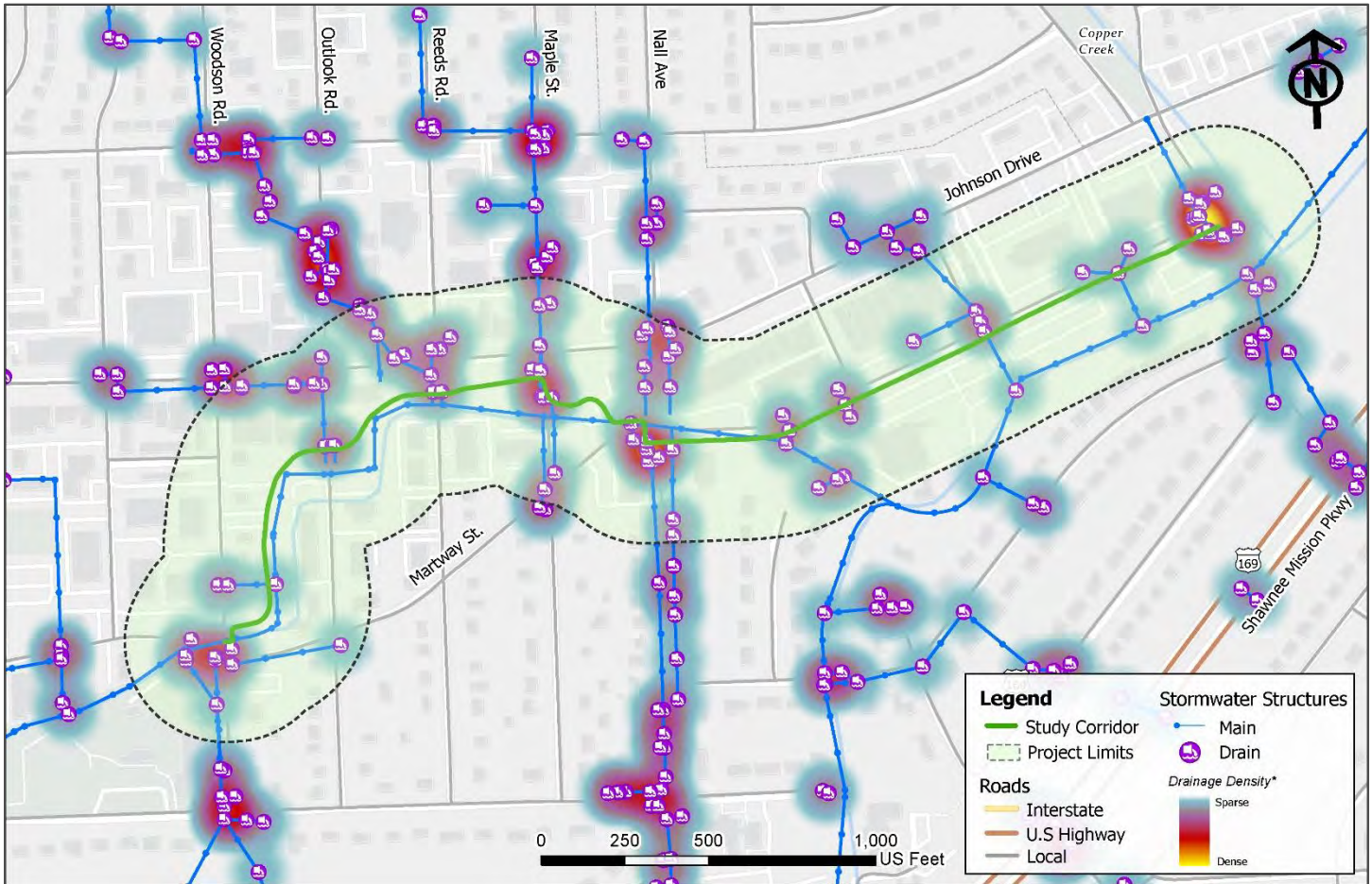
Figure 23 - Stormwater Drainage Density
