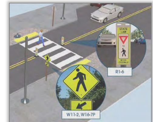
Figure 10 - High-Visibility Crosswalk (FHWA)
