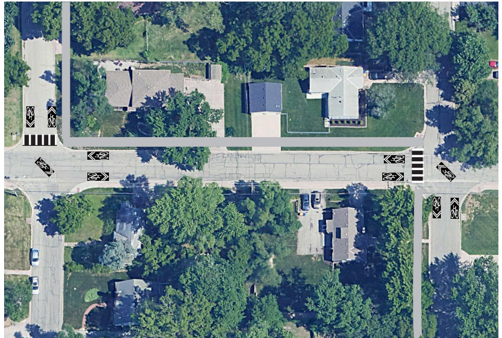
Negotiating jogs in the route. The Maple/Reeds bicycle boulevard includes several jogs because of disconnected or offset streets. These can be addressed through short sidewalk or sidepath segments on the busier connecting street and crosswalks. Shared lane markings can be used here to guide on-street cyclists through the jog.
